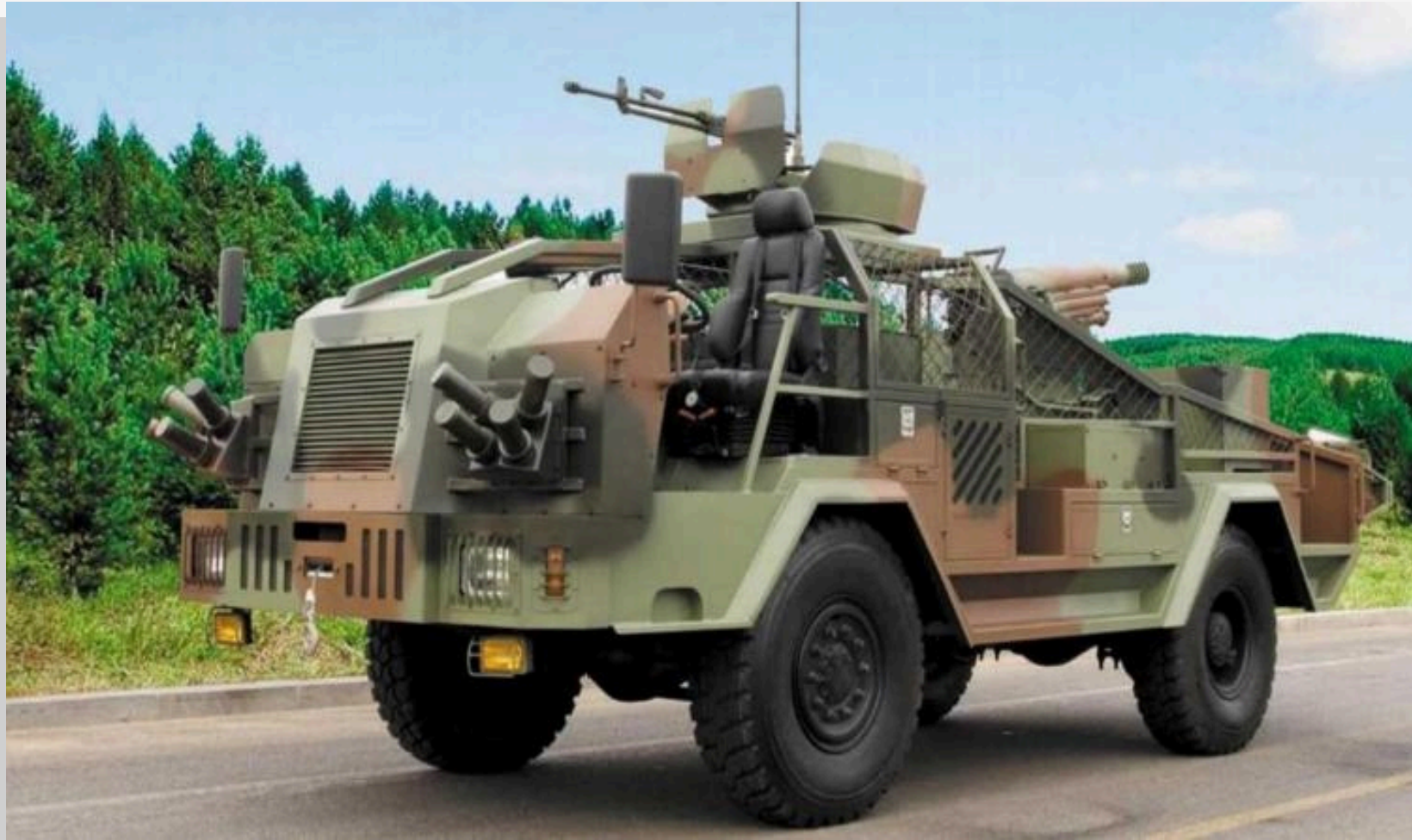
Tiansheng Supporting Vehicle Loaded with 105mm Rapid Fire Artillery
